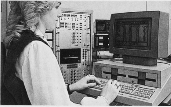
Fig. 152: Computer (photo from MSR [104]) to monitor final product specifications and quality trends of the final assembled relay as it comes off the production line
