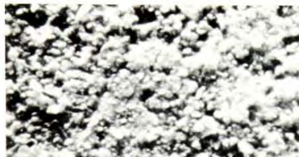
Fig. 85: Surface of a getter activated ferrite magnet (REM print \times 2600 enlargement)
