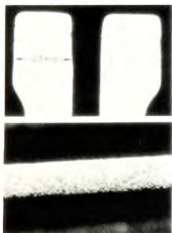
Fig. 86a: R-relay reed contacts (above) and fixed contact (below) in new state
