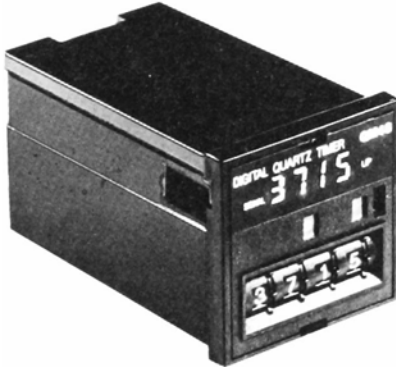
Fig. 159: Quartz controlled QM48 time-delay relay from SDS. Digital setting of required time and digital display of the actual time. Three time ranges 0.01 s to 100 s, 1 s to 100 min, 1 min to 100 h → relay tables
