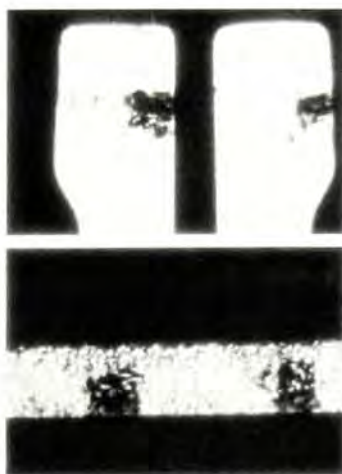
Fig. 86b: Ungettered R-relay reed contacts and fixed contacts after 52 \times 10^6 switching operations at 150 mV, 15 mA load
